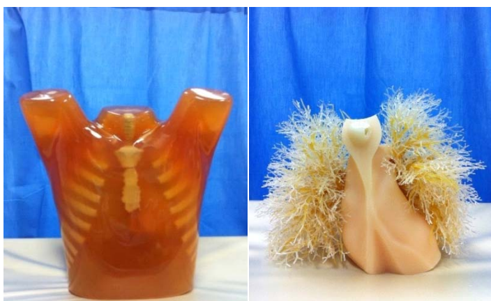
Figure 1. External (left) and internal (right) appearances of Lung man chest phantom.
