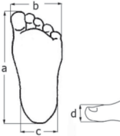
Figure 1. Four foot dimensions were measured: a. foot length; b. foot width; c. heel width; d. toe depth.
